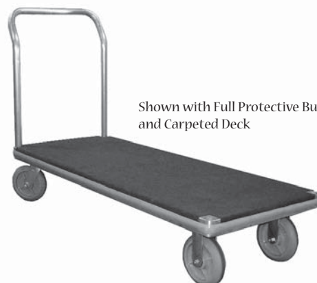
PT-3060S-150-850-C-310 30" x 60" smooth plate deck one standard #150 handle 8"x2" TPR casters (2 swivel, 2 rigid) carpeted deck full perimeter gray bumper 2,000 lb capacity
